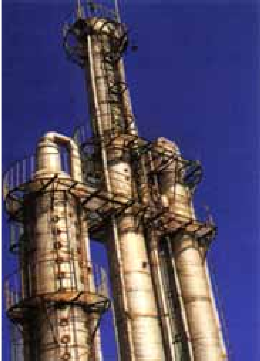
Six-tower differ-pressure distillation, Dukang Distillery, Henan
