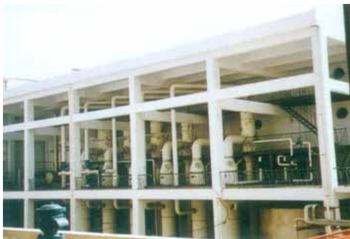
Six-effect evaporate and concentrate
