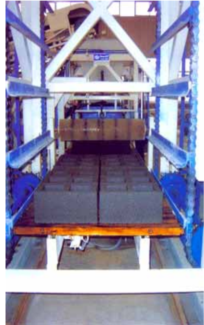
Elevator and lowerator system
