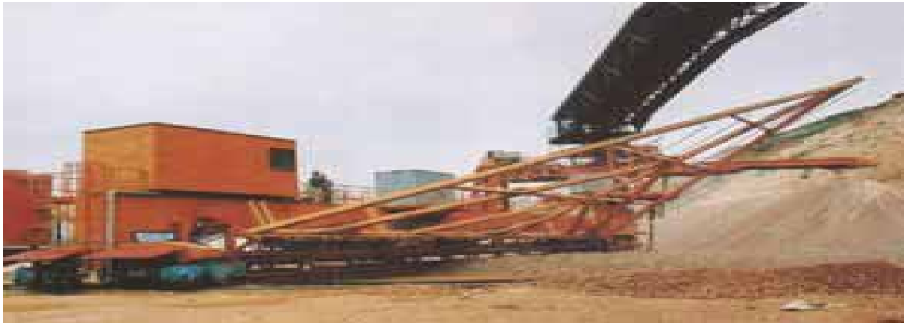
Stacker and reclaimer
