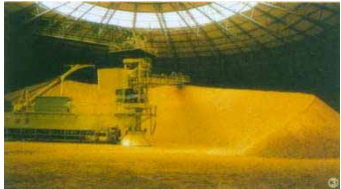
Homogenizing scraper stacker/reclaimer for circular stockyard (indoor)
