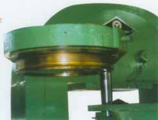
Sealing of the cylinder top
