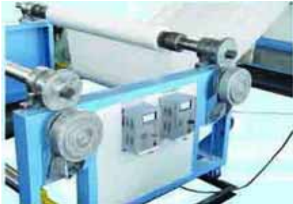
Automatic magnetism powder rises the control device of strength
