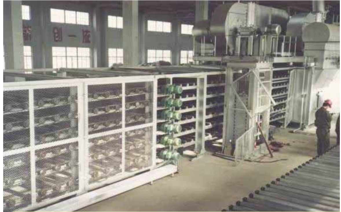
Open part of the dryer, and counter balance of the drive chain
