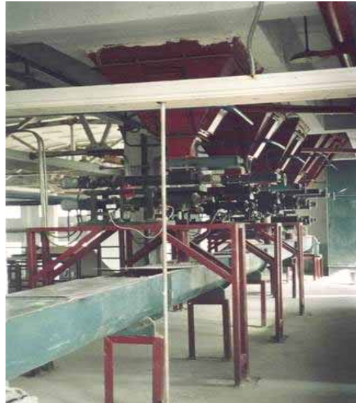
Electronic screw weigher for dosing
