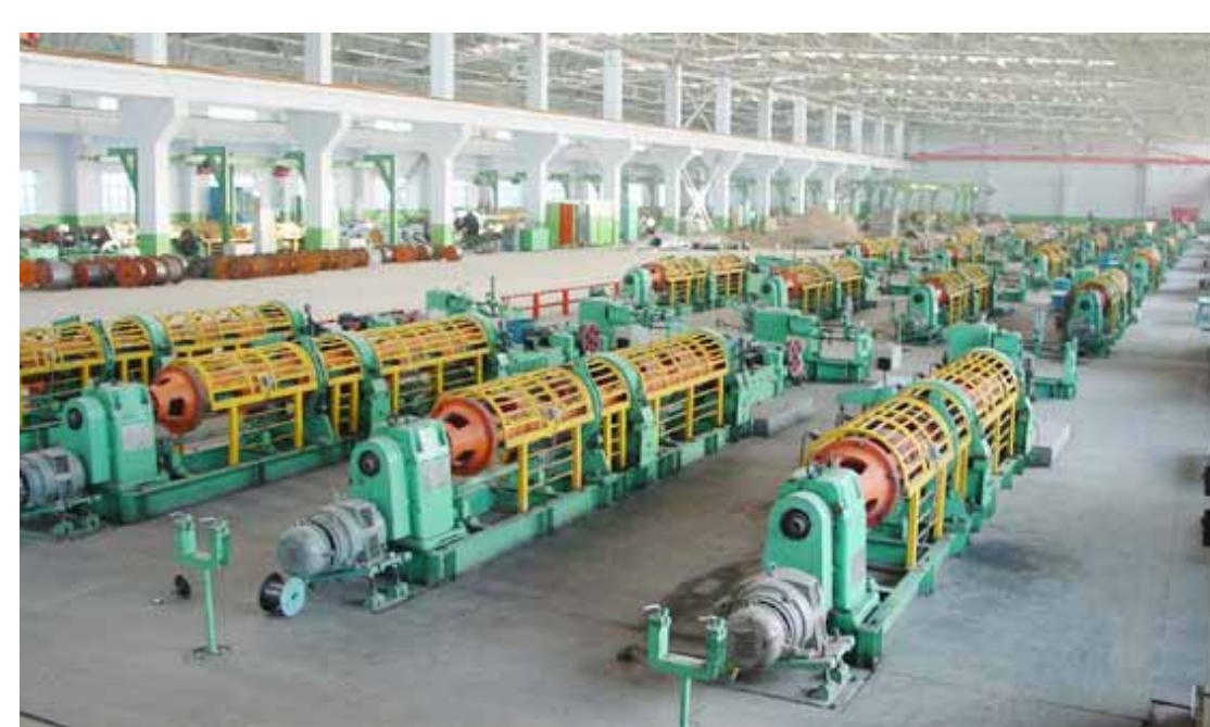
Stranding machine unit
